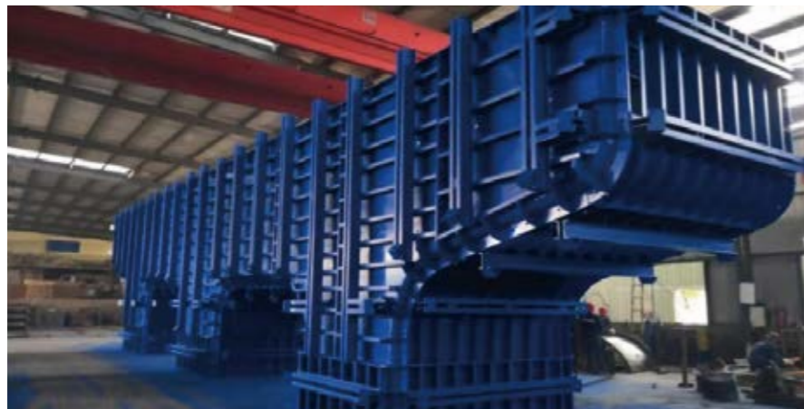
Steel Formwork for Bent Cap 盖梁钢模板
